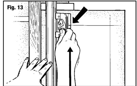
**Bevel Cutting Mat Openings Using Rail Stop**
