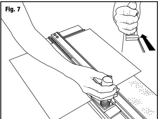
**Bevel Cutting Mat Openings, Without Rail Stops**
